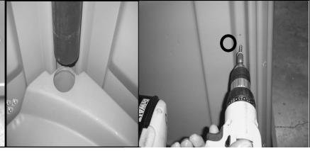
22) Drive 5th screw PN 13860 through rear panel into tank.
