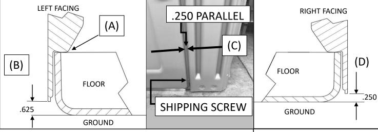
33) With the door screwed shut, transfer drill through [ 5 ] holes near the bottom of front facings, through floor using 5/16" (.312") [7.64 mm] drill bit. **NOTE**: *Insert .750* [19mm] thick block under facing if ground to facing gap is less than .625 [16mm].
