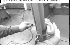
45) Place washer PN 12382 & nut PN 16307 on screw into recess of handle. Tighten screw/nut using # 3 Phillips Head Driver Bit & 7/16" (.437") socket. Tighten screw/ nut so handle is snug & not so loose that it could fall into closed position.
