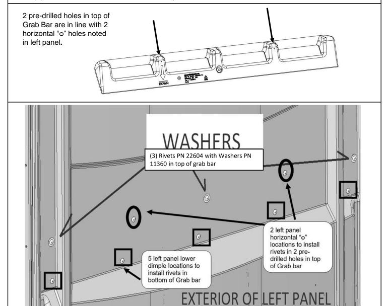
NOTE: INSPECT GRAB BAR INSTALLATION TO MAKE SURE ALL RIVETS ARE GRIPPING AND INSTALLED PROPERLY.
