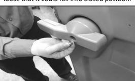
46) Handle when in open position, green color should be seen in indicator window of door. Red in color when handle is in closed position.
