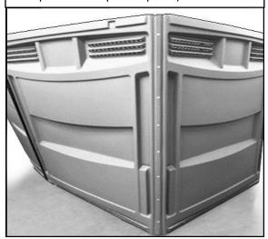
2) Use (8) rivets P/N 11054 & (8) washers P/N 11315 per corner.
