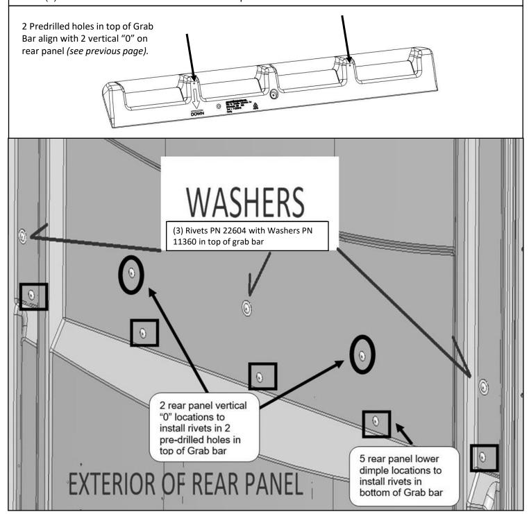
NOTE: INSPECT TGRAB BAR INSTALLATION TO MAKE SURE ALL RIVETS ARE GRIPPING AND INSTALLED PROPERLY.
