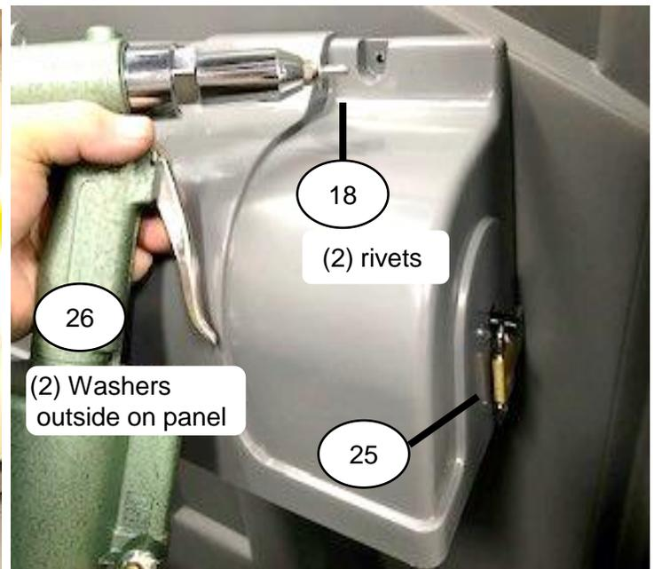
Install toilet paper rod #1051-699 in Paper guard hood from left to right end with hole in first. Place Padlock #1038-699 on end hole (out from right side of Paper guard hood). Fasten Paper guard hood to panel, use (2) Rivets #11054 inside through holes drilled in top of Paper guard hood into holes in panel & (2) Washers #11315 outside on panel.
