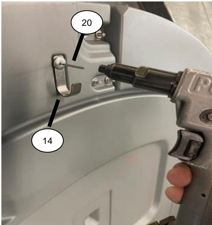
Drill dimple at top inside of front with #10 Drill bit. Rivet Coat #hook to front using rivet #22604.
