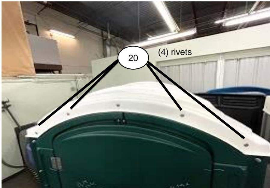
Finish fastening roof to front with (4) Rivets #22604.
