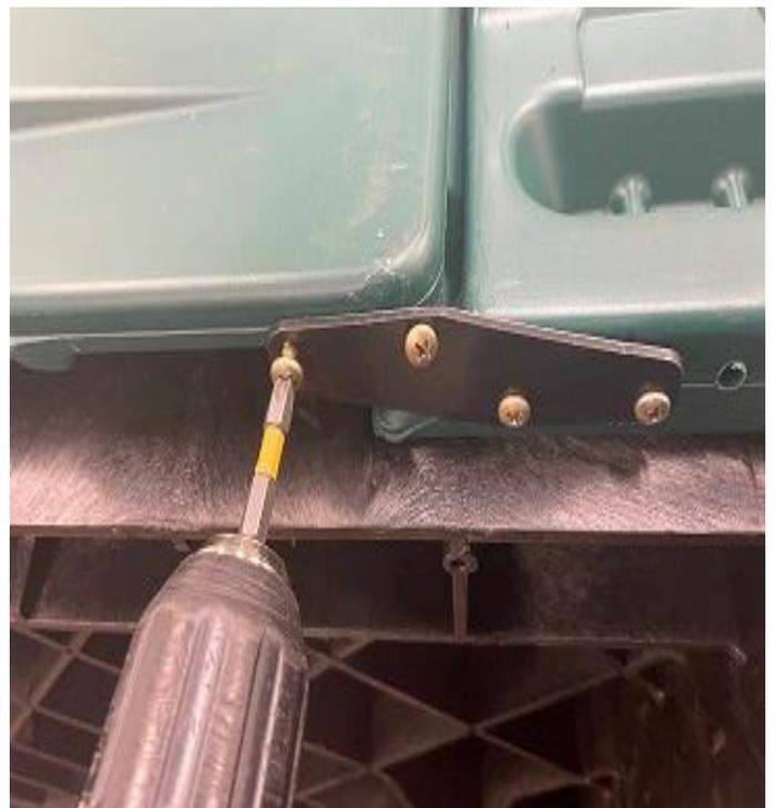
Install (2) Screws #13860 in holes on left & right side of front (door frame) at bottom, using a 3/8" or 5/16" Nut Driver bit **(DO NOT over tighten screws, run screws in until rubber washer begins to flatten).** Remove 4 screws in shipping strap at bottom of door & right door frame with Phillips driver bit.
