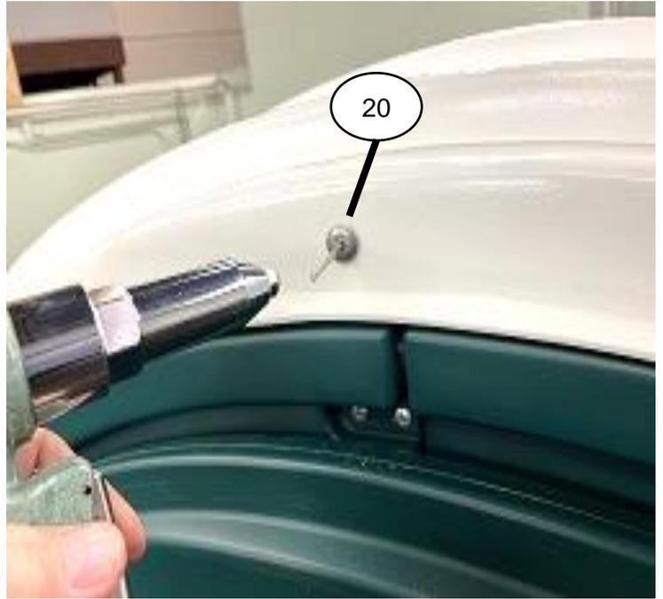
Push down on roof tight against front door frame. Transfer drill through 5 holes in roof through Front using #10 Drill bit .**Caution only drill through first wall of door frame.** Starting with center hole fasten Roof to Front with Rivets # 22604
