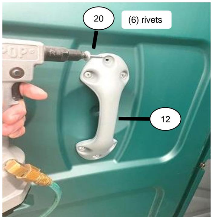
Rivet Handle #22522 to inside of door in 6 pre-drilled holes using rivet #22604.
