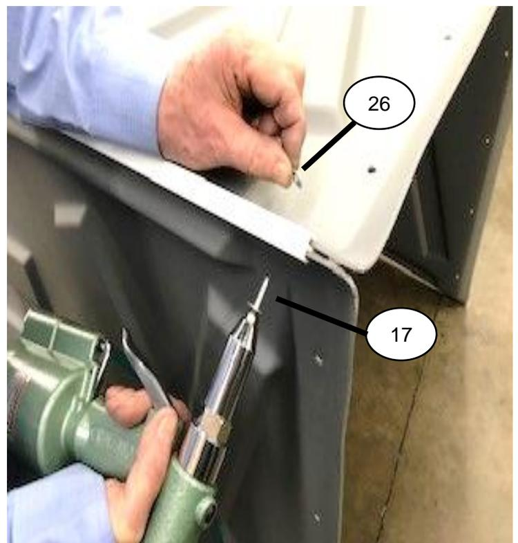
Fasten side panels to rear panel using (18) Rivets #11030 and (18) Washers #11315 (so rivet head is towards the front of unit & washer is towards rear of unit).
