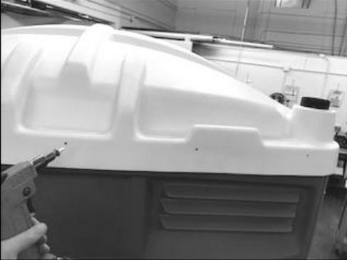
38) Rivet roof to rear panel using (5) rivets P/N 11054 installed from outside of roof & (5) washers P/N 11315 inside unit on rivets.
