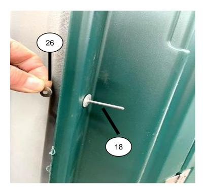
Tip unit up on base & place front against side panels with edge of panel tucked in groove on inside edge of front. Align holes in front with holes in panels & use 1 rivet #11054 on front & 1 washer #11315 on panel in middle in holes on left & right side of front.
