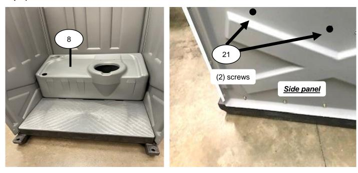
Place tank with seat area level when in base & down tight in base (*have someone sit on tank*). Locate 2 dimples in lower section of side panel as shown. Install (2) Screws #13860 through dimples into tank using 3/8" Nut Driver bit. Repeat sequence for other side panel. *(DO NOT over tighten screws, run screws in until rubber washer begins to flatten).*
