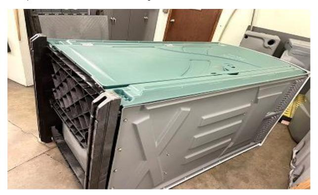
Tip unit onto rear panel & finish riveting front to panels using rivets (16) #11054 on front & (16) washers #11315 on panel.
